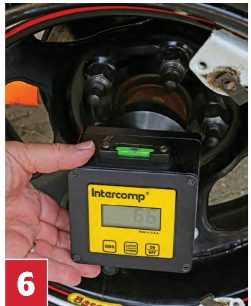
Switch the caster/camber gauge into camber mode. Straighten the wheels once again.
